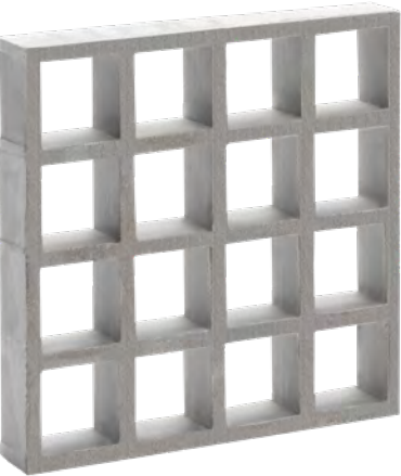
Gritted A non-slip gritted surface is obtained by applying sand to the concave-surfaced grating using a binding resin.
